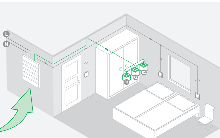
Example of a lighting system for controlling the light intensity by switching on sections R1 and R2 respectively
